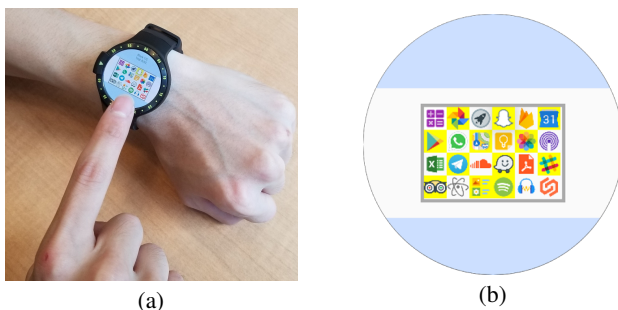
Figure 5. The setup of Experiment I. (a) shows a participant selecting a 4mm target, and (b) shows the application with 3mm square targets. The ones highlighted by yellow were the targets tested in the experiment.
